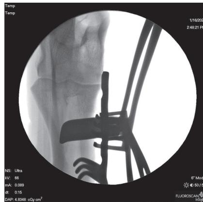
(Lower Left) Autofocus Image of Stainless-Steel Retractor Test Sample (66kV)
